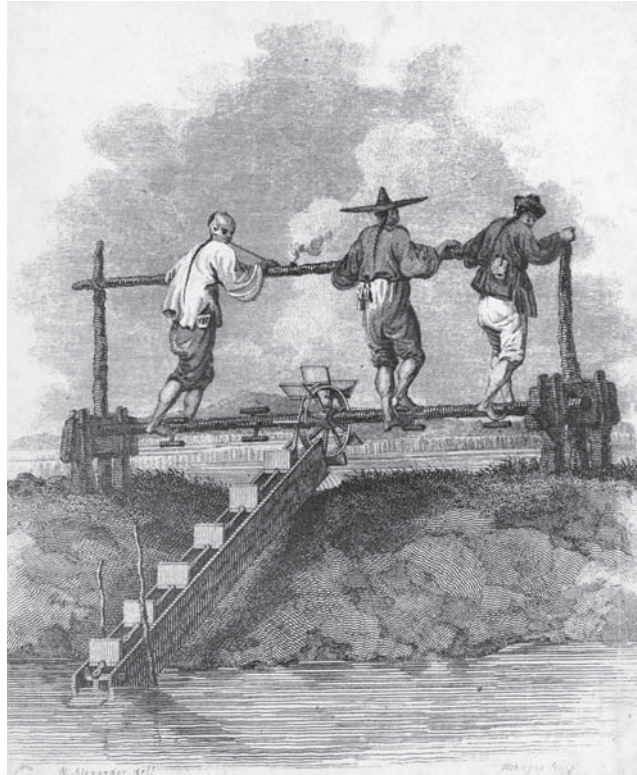
This late-eighteenth-century drawing depicts Chinese men treading the pole of a device that raises irrigation water. The men all wear the braided queue that Manchus required of Chinese men.
